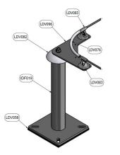
Rigging of a curved section on post
