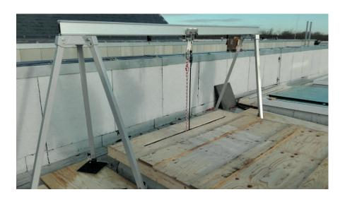
For an application in the construction industry, an anchoring device made by two tripods and a SafeAccess rail from which a RopeClimber bosun chair is suspended.
