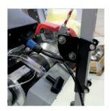
Detail RopeClimber fixing on tripod
