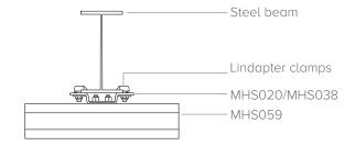
The adjustable brackets enable to:
