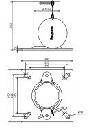
DAV008 Socket on roof height 500mm 17,5kg
