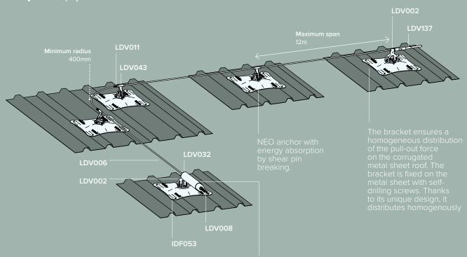
The energy absorber is a key component of an engineered cable lifeline. It reduces the forces transmitted to the host structure. Combined with the intermediate anchor LDV043 with integrated shock absorber, it enables the installation of the cable lifeline on a great variety of fragile roofs and structrures. The energy absorber has 4 functions: energy absorption in case of a fall, indicator of the tension in the line, upkeep of the tension in the line and indicator of a fall.
