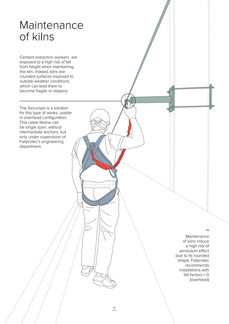
SecuRope lifeline between wall configuration with glider LDV133. For this type of configuration Fallprotec suggests the cable LDV005 construction 1x19 and Ø 8mm which reduces even more the deflection of the cable. Thanks to its properties it is also more resistant than others to
