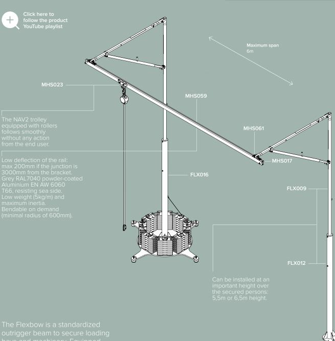
The Flexbow is a standardized outrigger beam to secure loading bays and machinery. Equipped with an integrated energy absorber, it is a lightweight and yet robust design for industrial applications with a minimum fall clearance of 4m. Several configurations (mobile, fixed on ground, fixed on wall ) are available
